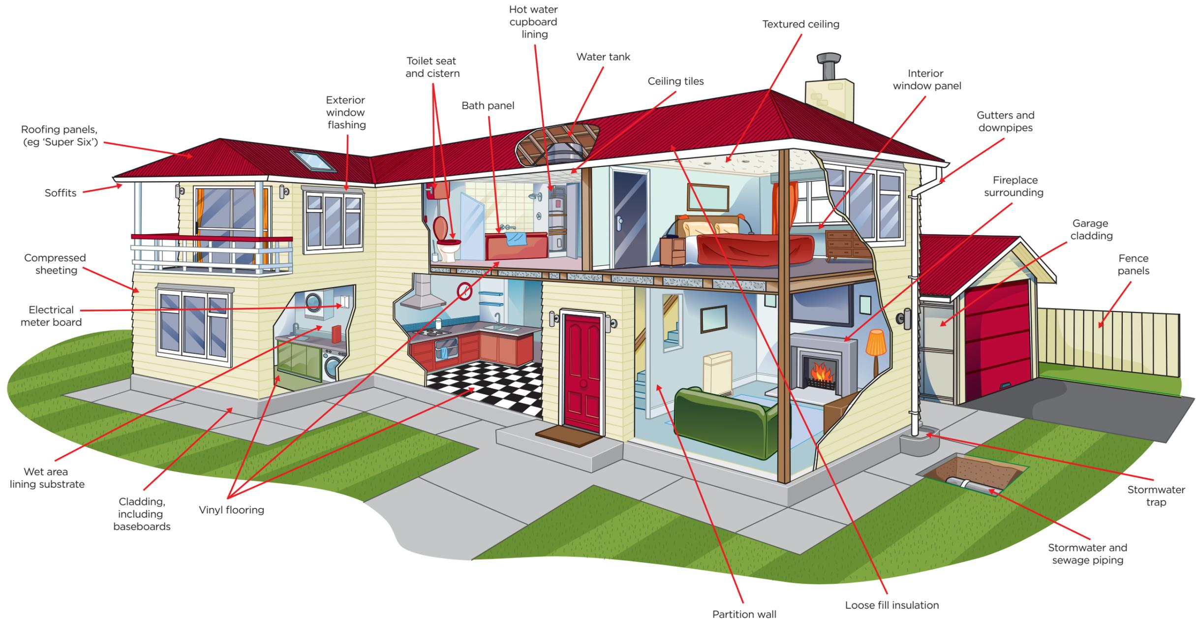
Buildings constructed before 2000 may have asbestos or asbestos-containing material (ACM). The diagram shows areas where asbestos or ACM were commonly used.
